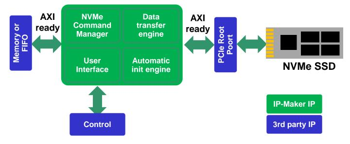
The architecture of the IP-Maker Host NVM Express IP is based on an AXI interconnect. It requires a simple engine (embedded CPU or FSM) for the configuration:
