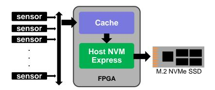
Using the pre-validated NVMe Host IP core greatly reduces time-to-market for storage OEM; this allows the OEM to benefit from a powerful data transfer manager. The IP-Maker Host NVMe IP core is full featured and easy to use in FPGA designs.
